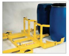
Designed for use with 210 litre Mauser open top and tight head egg shaped plastic drums. Arms close automatically around the base of the drum holding it securely during transportation. Fully automatic operation. Secured to the truck by fork pockets and screw clamps.
