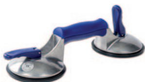
Aluminium body. Cap 60kg. Parallel lift. Slightly curved or textured surfaces.
