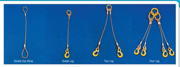
Wire rope slings by a British manufacturer to BSEN13414-1. All slings supplied with grade 80 rings, fittings and secured by mechanically spliced aluminium ferrules. Test certificate supplied. Capacity is nominal working load limit - in tonnes.
