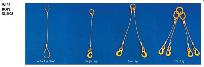
Wire rope slings by a British manufacturer to BSEN13414-1. All slings supplied with grade 80 rings, fittings and secured by mechanically spliced aluminium ferrules. Test certificate supplied. Capacity is nominal working load limit - in tonnes.
