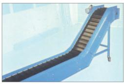
This flighted belt elevator has a simple modular framework construction, therefore it can be offered in a number of widths, heights and angles making it suitable for many applications. Can also be offered with a stainless steel framework
