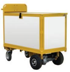
Full security cage fitted to platform. Infilled with heavy duty plastic formed sheet to avoid seeing contents.
