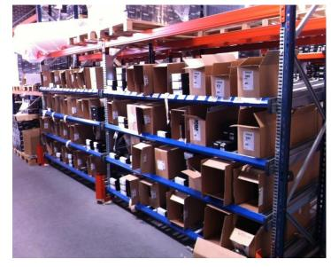
The Action Handling production team began to explore the best possible way to introduce a live storage rack system onsite, so components that were moving quickly could be picked and replenished efficiently and also free up dead space. Using the existing framework of the pallet beam racking we were able to install new live storage system and carry out "a very neat job" according to the client's production manager!
